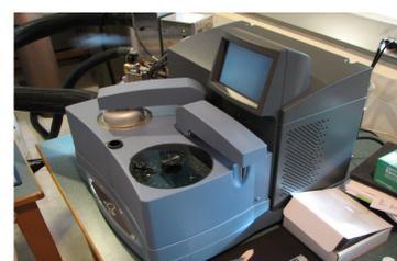
Figure 8: DSC Q2000 (TA Inst.) with modulated temperature control, autosampling robot, and LN<sub>2</sub> cooling system.
